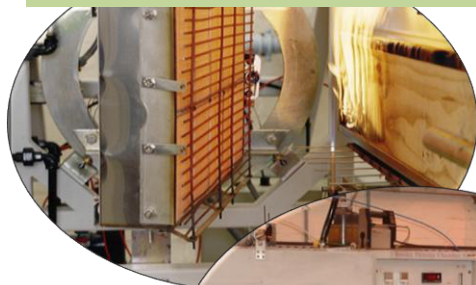
ISO 5658-2 "Flame spread test apparatus"
