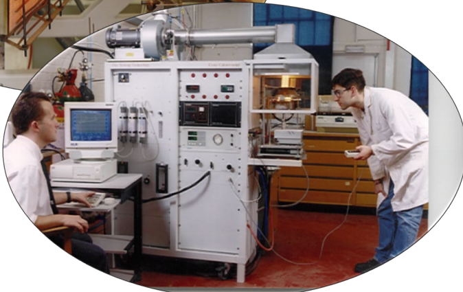
ISO 5660-1 Heat release rate test
