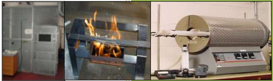
IEC 60754 tube furnace
