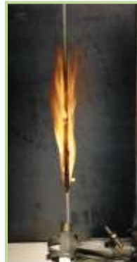
IEC 60332-1 vertical burn test
